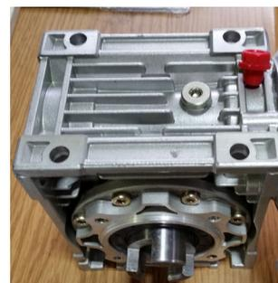
Diagram 6A. Installing breather on top of reducer.
