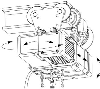
**Figure 39:** Movement between chain hoist and trolley.
