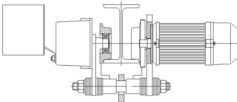
**Figure 32:** Counterweight for electric trolley.
