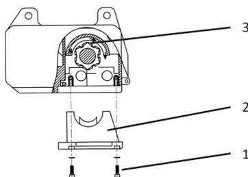
**Figure 43:** Removal of the chain guide.
