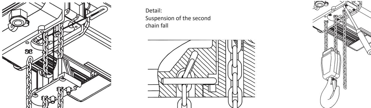
Figure 50: Fixation of the second chain fall to the hoist body.
