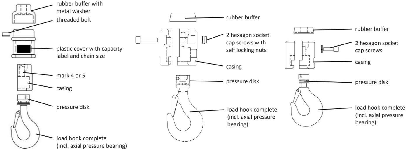
Figure 40: Details of the bottom hook - single fall.
