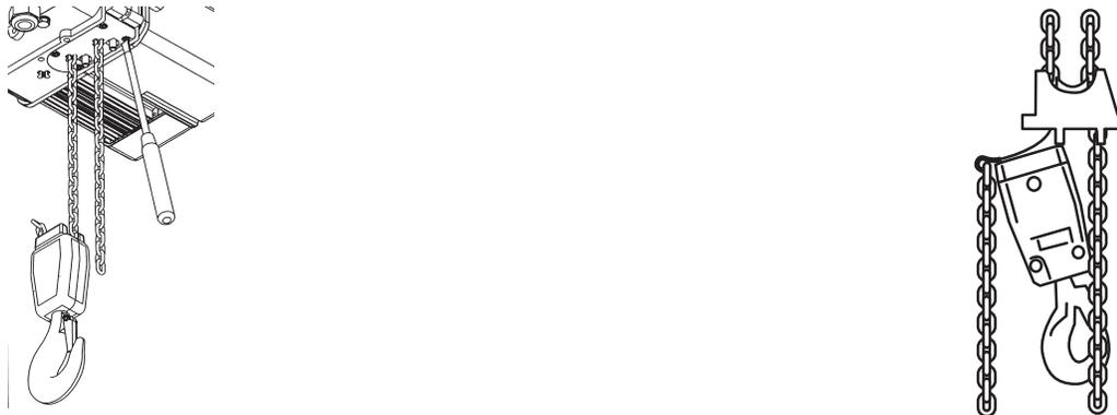
Figure 49: Completion of double fall version.
