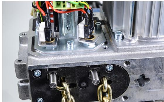
Figure 29: Electric limit switches for low voltage control.
