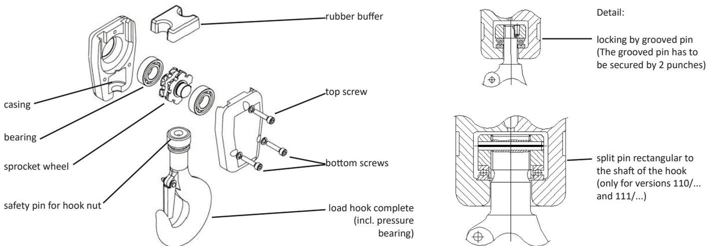
Figure 41: Details of the bottom hook - double fall.
