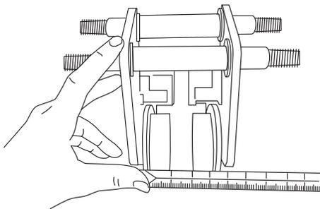
Figure 35: Determination of quantity of washers.
