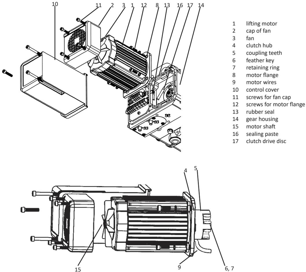
Figure 52: Dismantling and assembly of the lifting motor.
