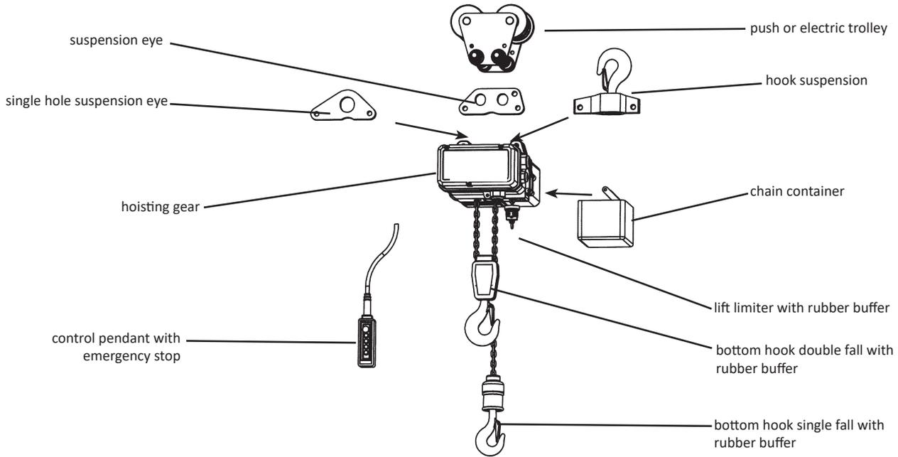
**Figure 3:** Electric chain hoist and its accessories.
