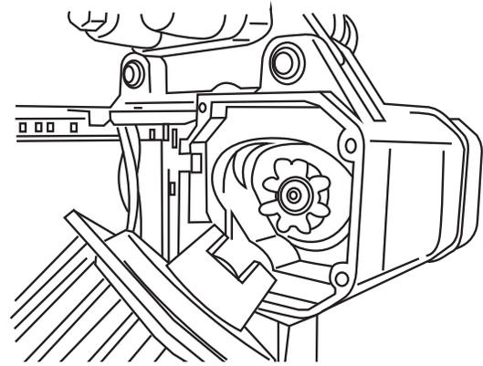
Figure 55: Dismantling the motor.
