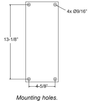
**3a.3** Lift boom assembly up and bolt lower and upper bearing mounts to support structure using  $\text{Ø}1/2$ " bolts Grade 5 or better.
