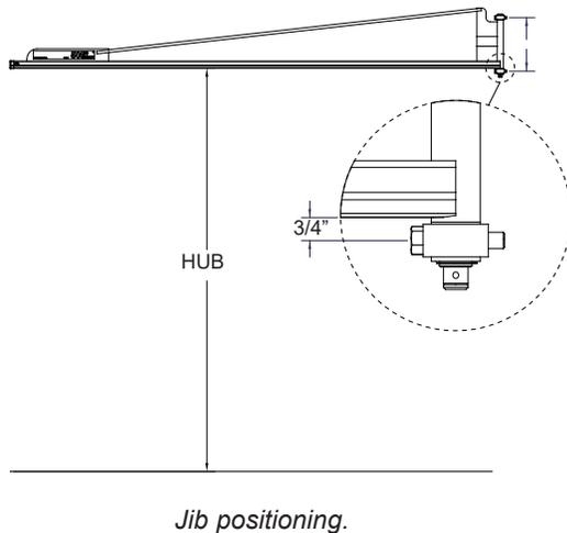
**3a.2** Drill bolt holes and bolt **lower** pivot mounting assembly to support structure.
