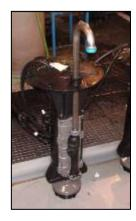
When assembly of the grinder pumps is complete, they are moved by conveyor to the final inspection station. At this work cell, an operator moves the core from the conveyor to a water tank where it is fully submerged in water and connected to a diagnostic machine. Full functionality of the core is tested here in about three minutes, after which they are removed from the tank, drained, and either approved for shipment or rejected for failing one of the critical tests.
