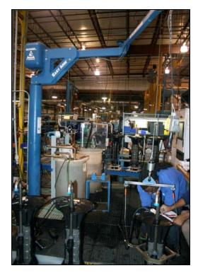
With the release of a new series of the grinding pumps, the company needed to create an additional inspection station to increase the number of pumps it could inspect in a day. In the existing work cell, a floor supported bridge crane covers the entire work area and features a large manipulator to assist in lifting the pump cores and placing them into the water tanks.
