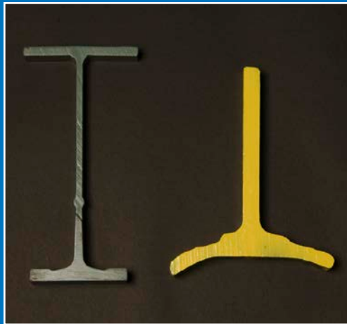
Peening caused the mild steel flange on this I-beam to bend, making it completely unsafe for crane travel.
