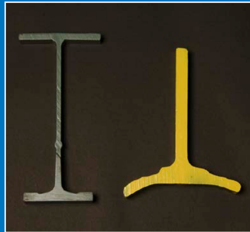
Peening caused the mild steel flange on this I-beam (on right) to bend, making it completely unsafe for crane travel.
