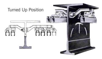
Steel brackets, which mount directly on the track web, support conductors on 10" and larger patented track. These supports can be turned up or down, depending on track depth and wheel size. One to six conductors can be held by the off-web supports.
