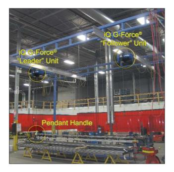
With G-Sync<sup>™</sup> Technology, the operator is now able to lift the long metal trays pictured at right by attaching both G-Force<sup>®</sup> units to either end. By controlling the lift from one pendant handle, the operator safely lifts the load in one synchronized motion which keeps the load balanced and easy to position on shipping carts.
