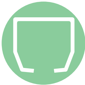
2-degree taper keeps the trolley centered
