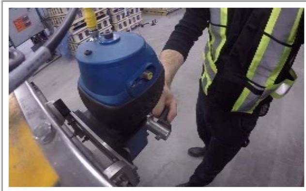
coating line using the Gorbels G-Force®. The bin foundation is lifted from a stack and then hung on hooks suspending the product as it goes through the line. At the end of the line the product is removed from the hooks and stacked using the same G-Force® handling device.
