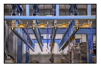
At this manufacturer, the interlocks are needed to transfer product in and out of the paint system. The products vary greatly, from batches of small flat bar washers to structural steel columns, channels and beams. The weights can run from hundreds of pounds to a couple thousand pounds per monorail. The operator hangs the products along the bridge and transfers it into and out of each paint system booth.
