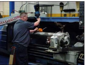
The original G-Force® installed was a 1320 pound capacity Q model with Float Mode and a high capacity magnet to grip parts. The G-Force® was installed onto an existing Gorbel work station crane with a 2,000 pound capacity aluminum bridge. It is used to the final process in assembling hydraulic cylinders that measure 8 to 10 feet long and weigh over 1,000 pounds.
