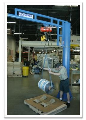
In the printing area, the customer selected a 1000 pound capacity freestanding work station jib crane with 360 degree rotation, an 8 foot span and 10 foot height under boom along with an electric chain hoist. The Gorbel jib
