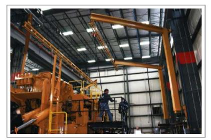
In order to provide the most fall protection coverage without obstructing the crane movement, they installed four Tether Track fold away fall arrest systems. The systems feature dual track rails so that each track can support two workers. Two of the systems are 100' long and two are 150', and they are supported every 50' by wall cantilever style jibs. One jib per Tether Track system is motorized so that it can either be easily positioned at any point in the jib's
