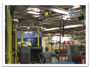
"We had a lot of in-house built, I-beam type bridge cranes and Spanmaster I-beam jib cranes, but we were having a lot of trouble." The heavy I-beam style cranes were very bulky and hard to move, and didn't offer Snap-On much flexibility for future changes.
