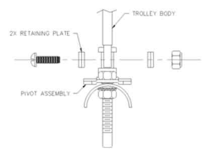
2. Tooling may now be hung or bolted to the trolley plate without interference.
