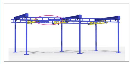
Gorbel® Maintenance Gates make it easier to service systems with 3 or more bridges, like this one, by giving you access to inside bridges without having to remove the outer bridges.
