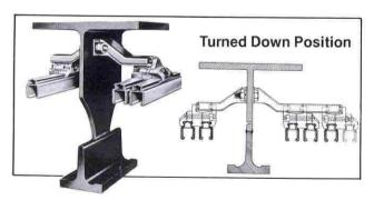
Steel brackets, which mount directly on the track web, support conductors on 10" and larger TARCA Track. These supports can be turned up
