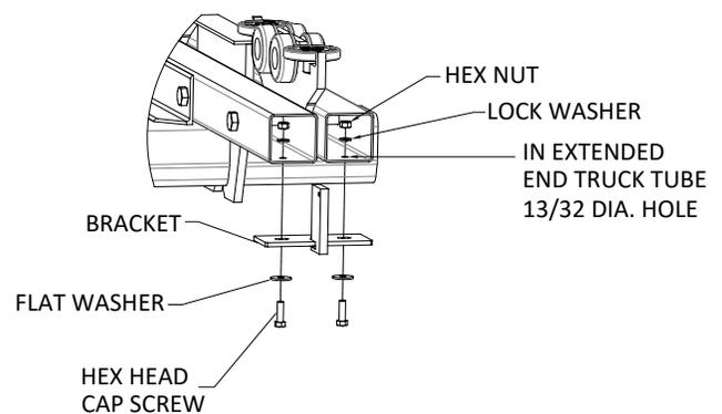
**Diagram 3B.** Extended End Truck Mounting Bracket.
