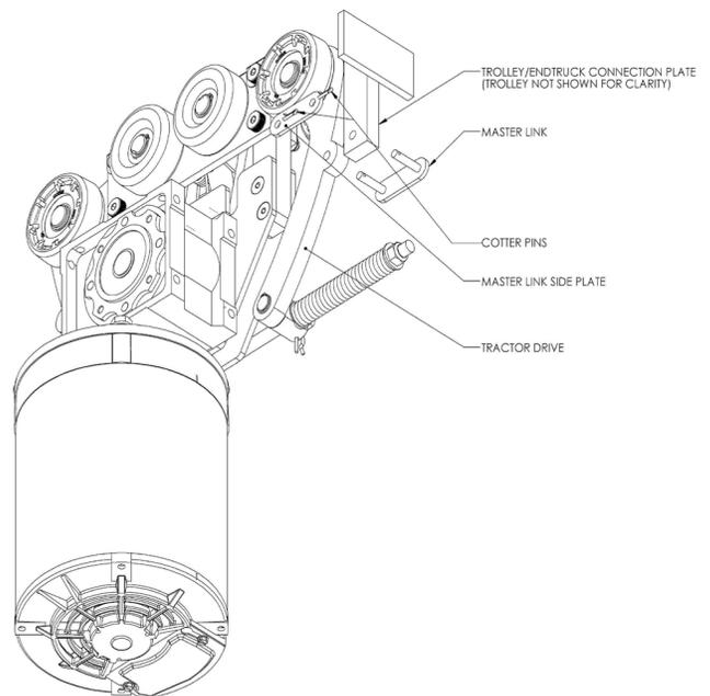
Diagram 6A. Link Pin Installation.
