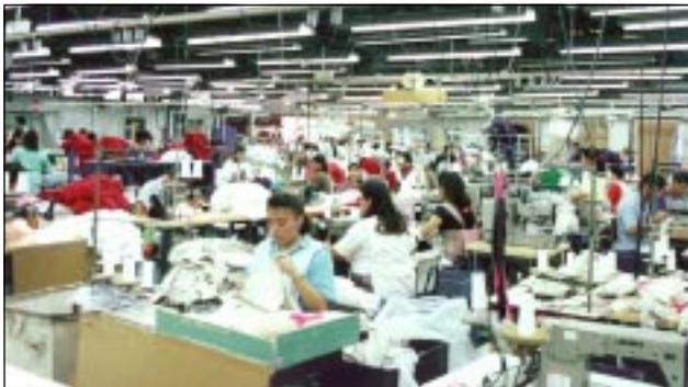
Sewing rooms use stationary Power Jacks which plug into the Four-Bar runs overhead. Machines can be added or relocated quickly and easily.
