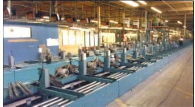
Another appliance manufacturer has 166 moving carriers for evacuation and burn-in testing on a loop. Another brand of conductor rail was replaced after giving trouble ever since it was installed. Four-Bar has operated with total satisfaction.
