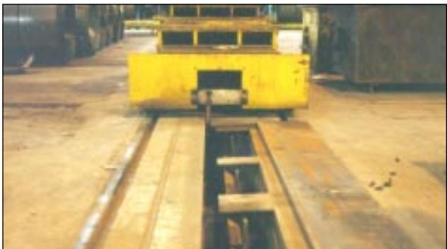
This trench-mounted Tri-Bar withstands dirt, oil and moisture to electrify a steel coil transfer car.
