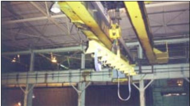
Four-Bar is used on the bridge of this crane for main power and control lines.
