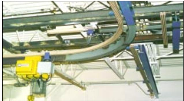
Four-Bar is perfectly formed to any curve, switch and transfer requirement. Systems are custom fabricated to customer requirements.
