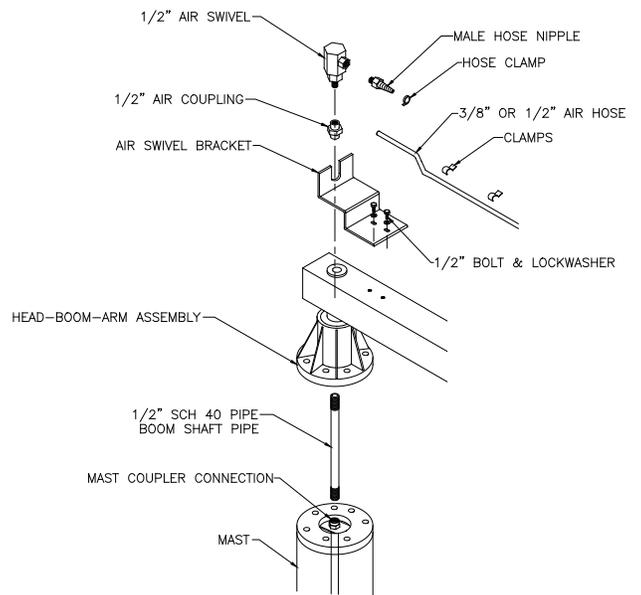
**Diagram 4D.** Boom bottom entry air swivel assembly.
