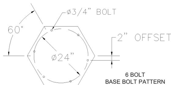
Diagram 2E. Baseplate dimensions for 8-5/8" and 12-3/4" masts.
