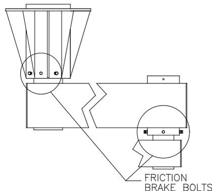
Diagram 2B. Friction brake bolt location.
