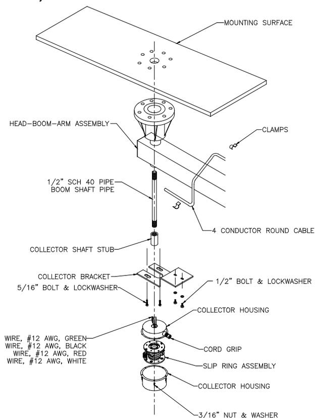
Diagram 3C. Boom Electrical Bottom Entry Collector.
