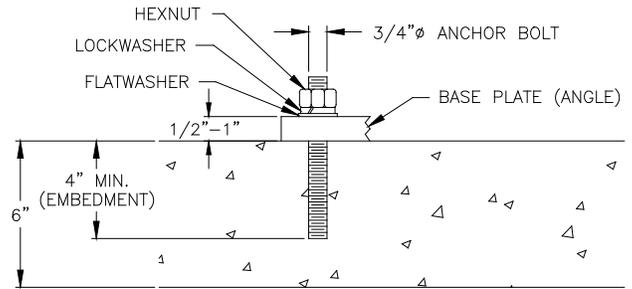
**Diagram 1A.** Typical anchor bolt embedment.
