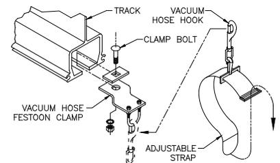
Diagram 8C. Installing vacuum hose clamp on runway or bridge.
