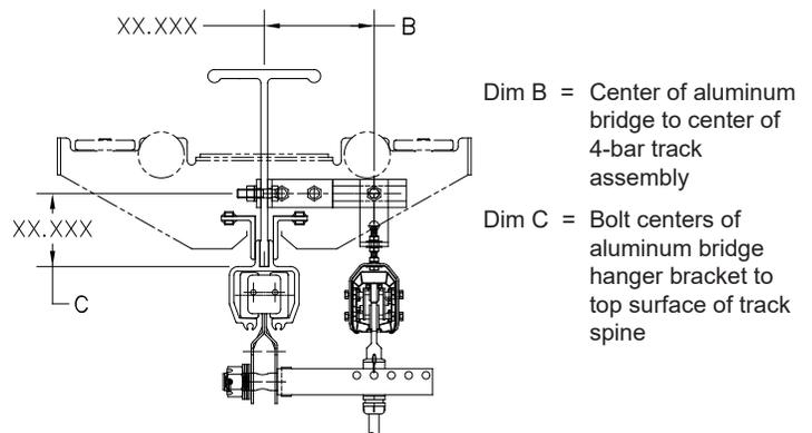
**Diagram 10F. Two piece aluminum bridge B-C dimensions.**
