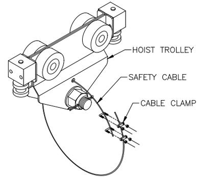
Diagram 6H. Installing safety cable on hoist trolley.
