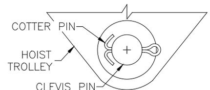
Diagram 6M. Installing cotter pin through trolley clevis pin.
