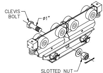
Diagram 6L. Installing hoist on A2000 loadbar hoist trolley.
