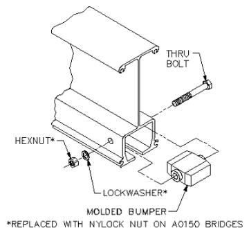
Diagram 8D. Installing endstop on runway/festoon stack section.
