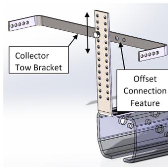
**Diagram 10L.** Tow bracket directly mounted to mast.
