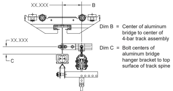
**Diagram 10E. One piece aluminum bridge B-C dimensions.**
