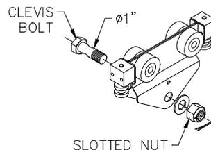
Diagram 6K. Installing hoist on A1000-A2000 hoist trolley.
