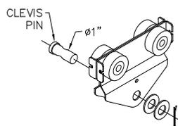
**Diagram 6C.** Installing hoist on A1000-A2000 hoist trolley.
