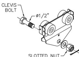
**Diagram 6A.** Installing hoist on A150 hoist trolley.
