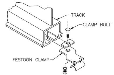
Diagram 8B. Installing clamp on runway or bridge.
