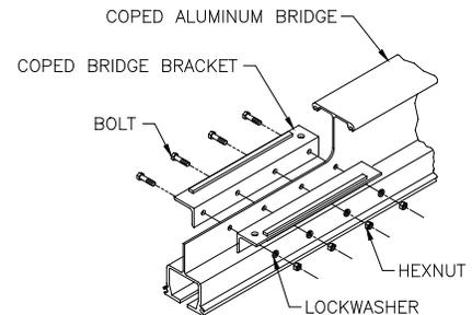
**Diagram 5B.** Installing brackets on coped/two-piece aluminum bridge.
