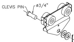
**Diagram 6B.** Installing hoist on A250-A500 hoist trolley.
