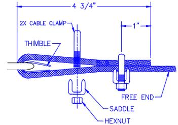
**Diagram 9D.** Saddling the cable on one end.
