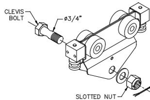
Diagram 6J. Installing hoist on A250-A500 hoist trolley.
