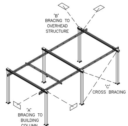
**Diagram 1.** Examples of typical sway bracing locations.
