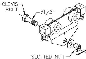
Diagram 6I. Installing hoist on A150 hoist trolley.
