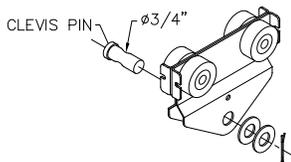
**Diagram 6B.** Installing hoist on A250-A500 hoist trolley.
