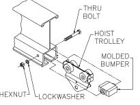
Diagram 3H. Installing hoist trolley and endstop.
