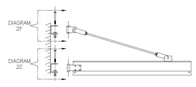
Diagram 2G. Attaching aluminum jib to formed channels.
