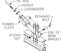
**Diagram 2C.** Bolting end of beam bracket to boom.
