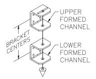
**Diagram 2A.** Plumbing formed channel brackets.
