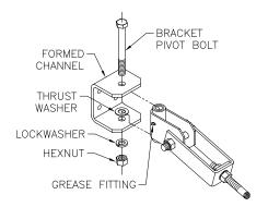
**Diagram 2F.** Attaching upper pivot assembly to upper formed channel.
