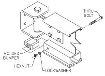
Diagram 3A. Endstop installation.
