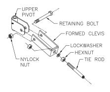
**Diagram 2D.** Attaching upper pivot assembly to tie rod.
