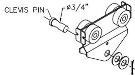
**Diagram 3D.** Installing hoist on A250-A500 hoist trolley.
