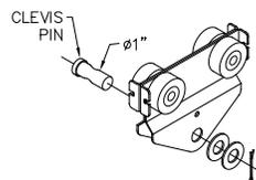
**Diagram 3E.** Installing hoist on A1000 hoist trolley.
