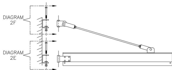
**Diagram 2G.** Attaching aluminum jib to formed channels.
