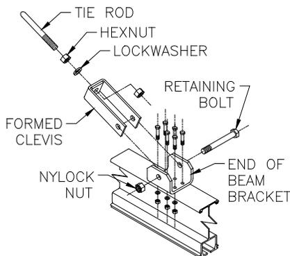
**Diagram 2C.** Bolting end of beam bracket to boom.
