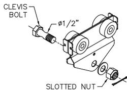
**Diagram 3C.** Installing hoist on A150 hoist trolley.
