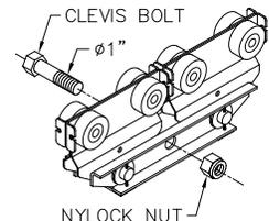
**Diagram 3F.** Installing hoist on A2000 hoist trolley.
