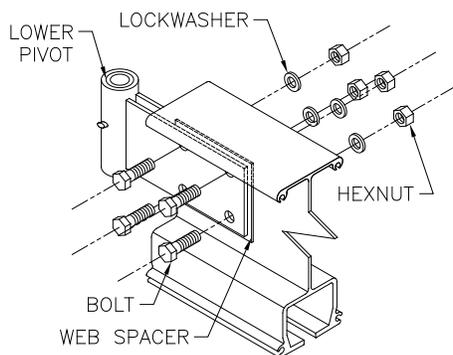
**Diagram 2B.** Bolting lower pivot assembly to boom.
