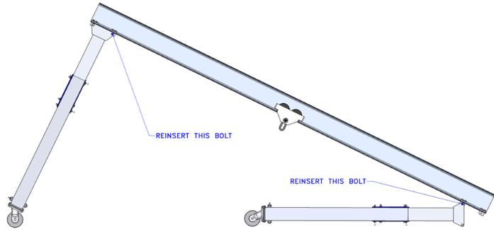
**2.5** Position second leg under partially erect gantry (**diagram 2C**) and install one bolt and nut through leg gusset plate and pivot tube. Finger tighten nut.
