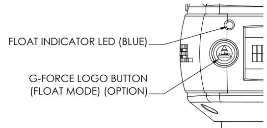
**Diagram 12A.** Float Mode Button - Slide Handle.
