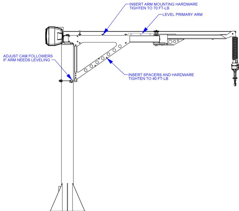
Diagram 4B. Arm assembly-leveling adjustment.
