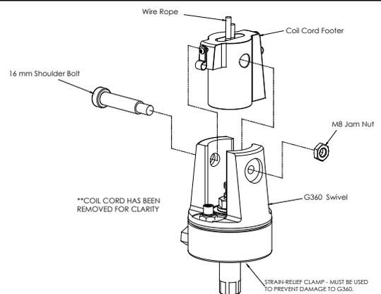
**Diagram 6B1.** G360™, Shoulder Bolt and Coil Cord.
