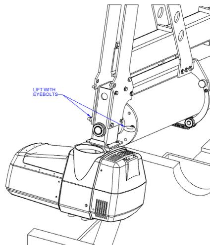
Diagram 2E. Easy Arm® assembly removal from packaging.
