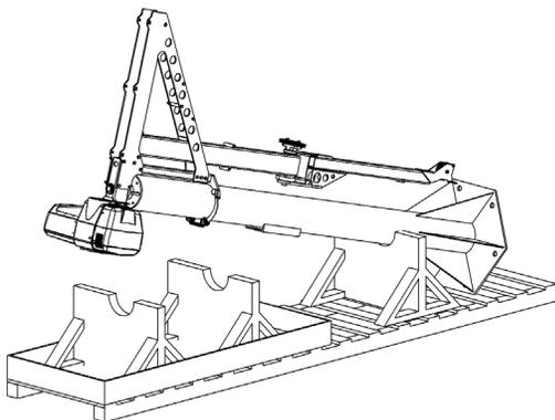
Diagram 2D. Easy Arm® assembly removal from packaging.
