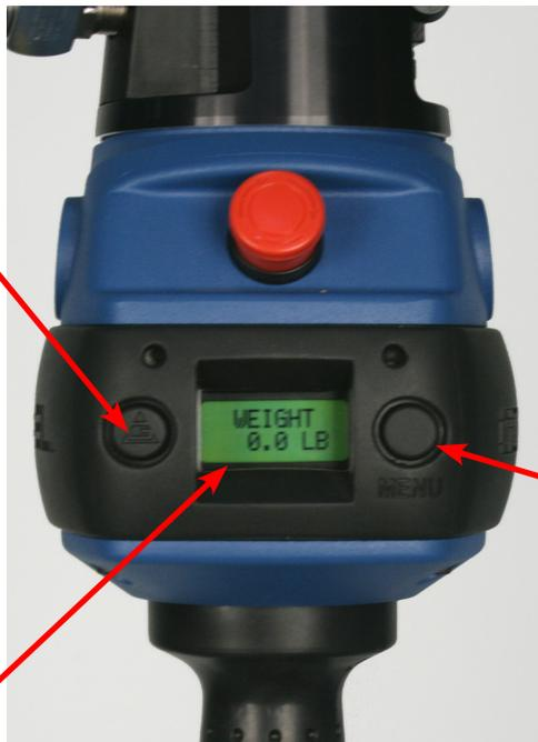
Press and hold this button for approximately three seconds until the unit enters program mode. Once in program mode, this button is used to select the desired menu. Press and release this button to advance to the next menu. If you happen to accidentally pass by a menu, it will come around again if you continue to press and release this button.
