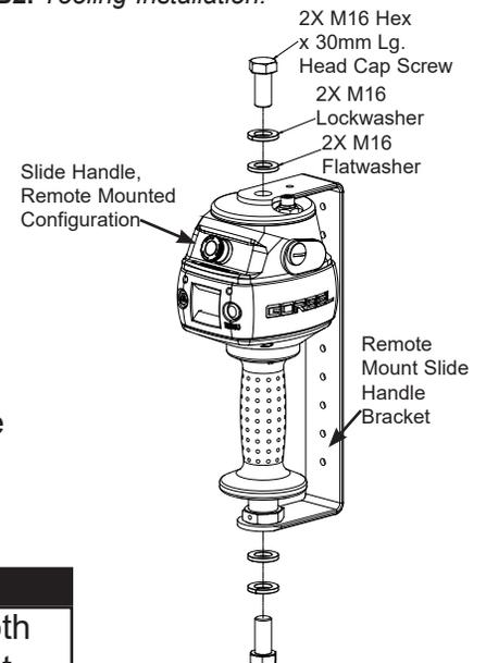
**Diagram 6B3. Remote Mounted Slide Handle, Exploded View.**
