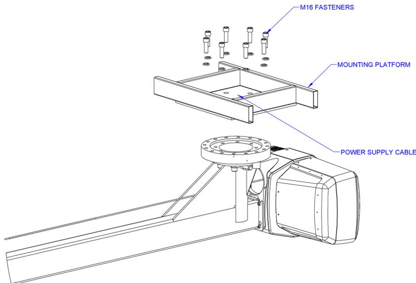
Diagram 5A. Installing Under Hung Easy Arm®.
