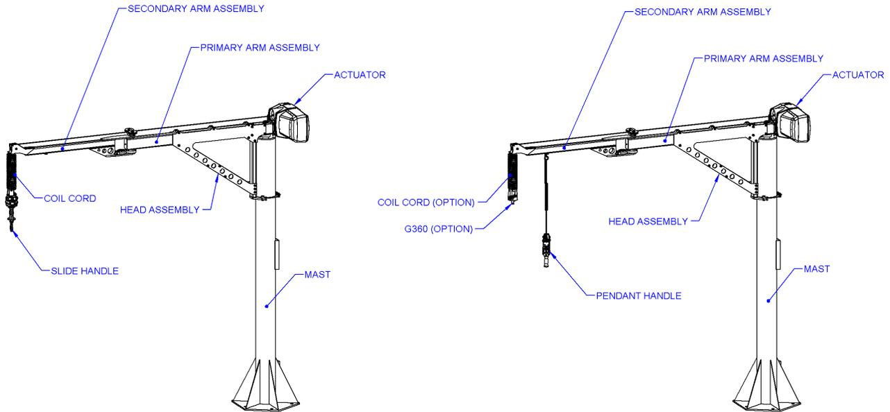
Diagram 1A. Main Floor Mounted Easy Arm® Components.
