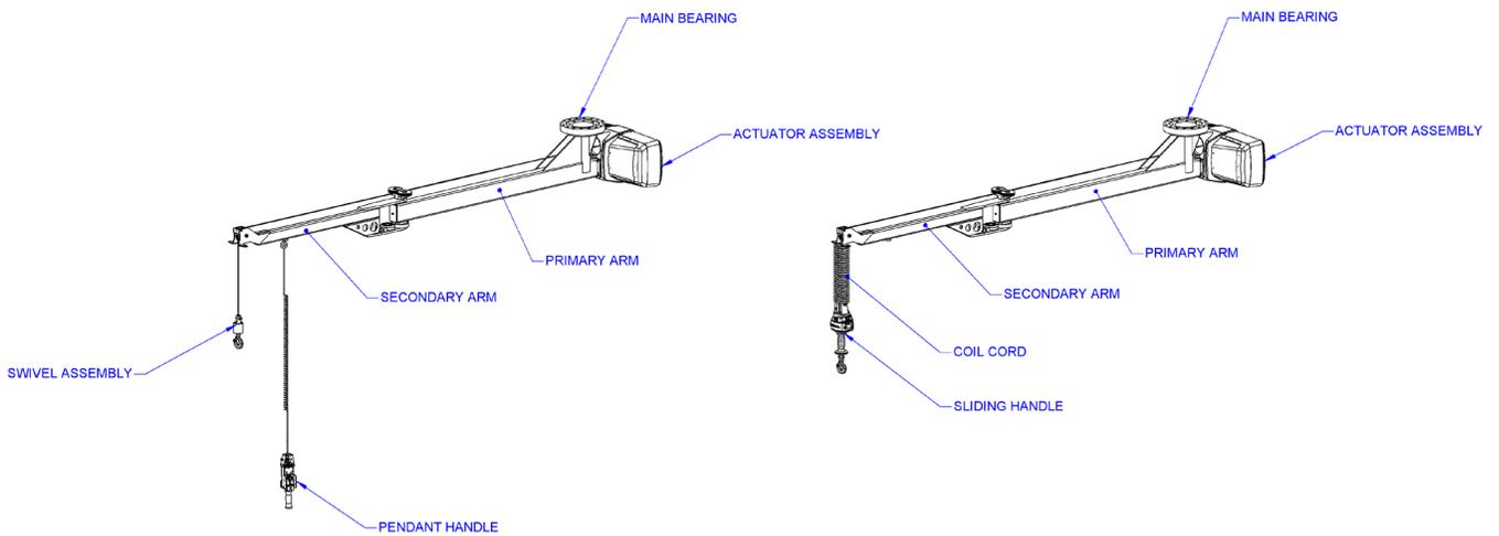
Diagram 1B. Main Under Hung Easy Arm® Components.
