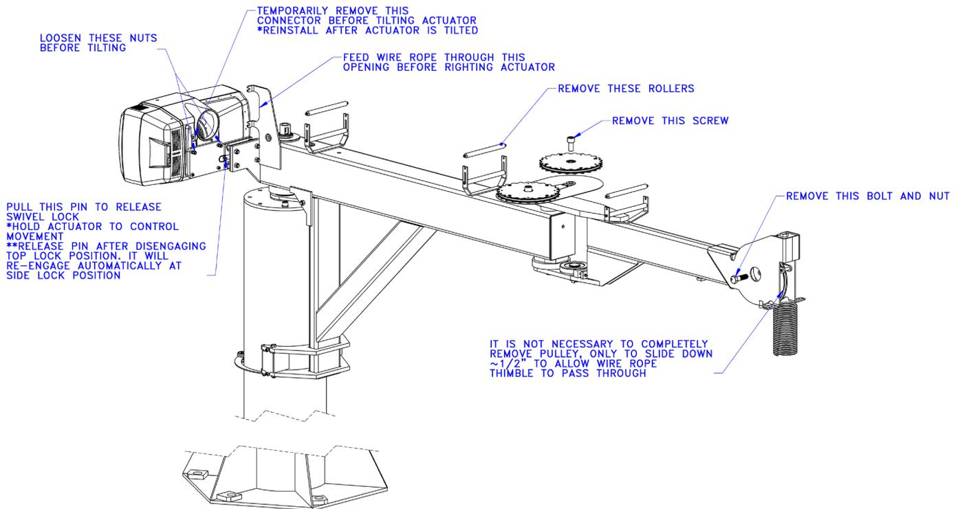
Diagram W. 660# Easy Arm wire rope replacement.
