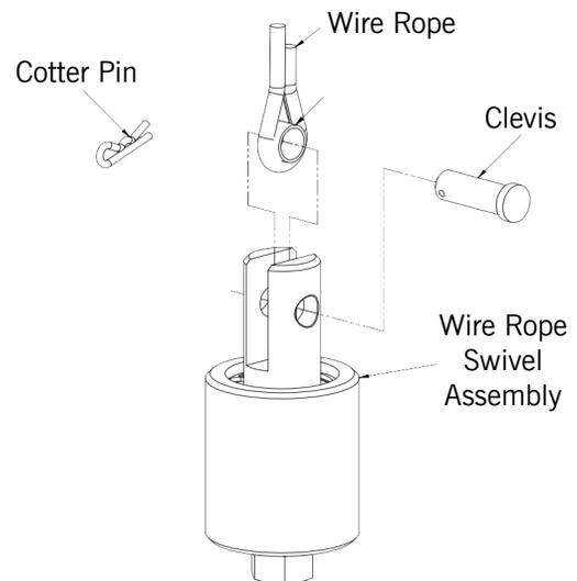
**Diagram 7-3.** Removing the Wire Rope from the Pendant Handle.
