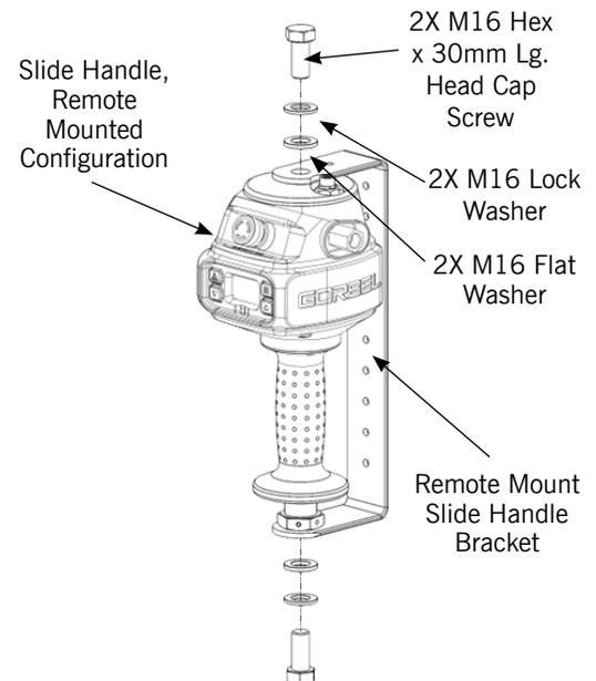
**Diagram 2-21.** Remote Mounted Slide Handle, Exploded View.
