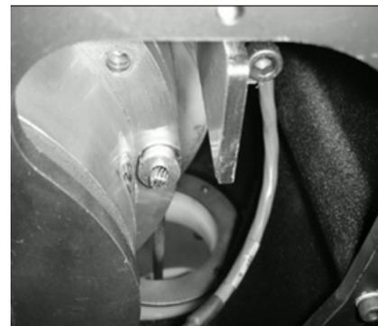
**Diagram 7-9.** Wire rope crimp fully seated in recess.
