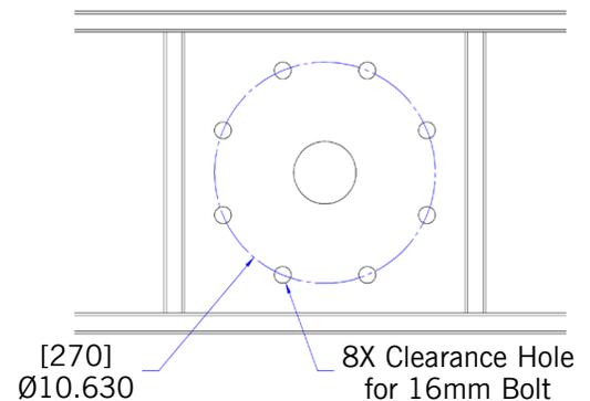
**Diagram 2-16.** Bolt Pattern for Under-Hung Easy Arm.
