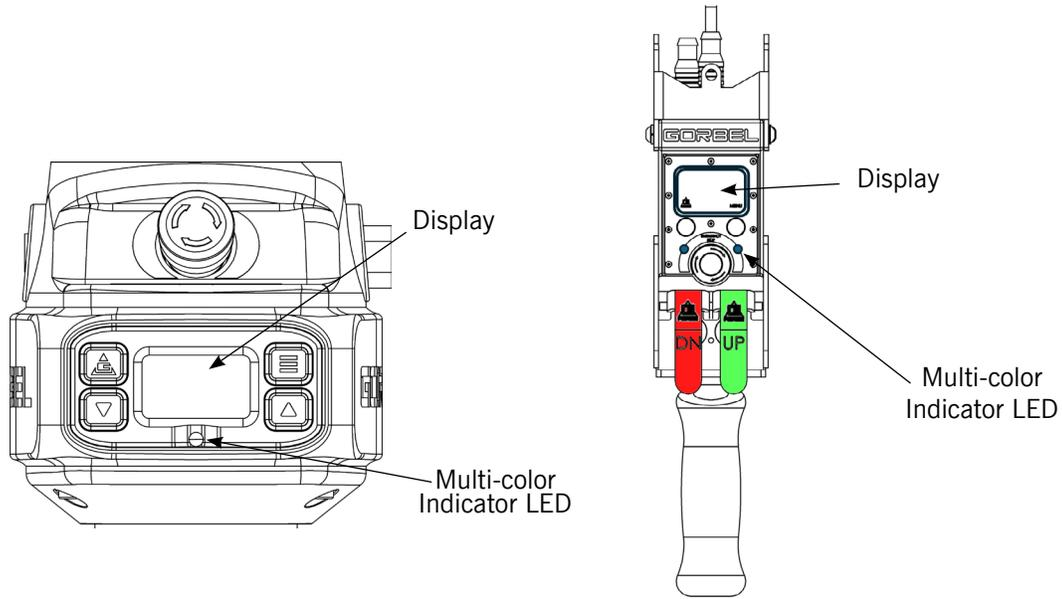
**Diagram 5-1.** Slide and Pendant Handle Displays and LEDs.
