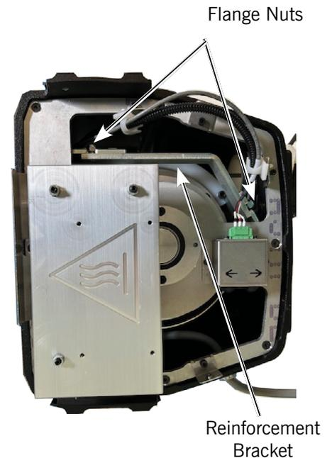
**Diagram 7-4.** Flange Nuts and Reinforcement Bracket.
