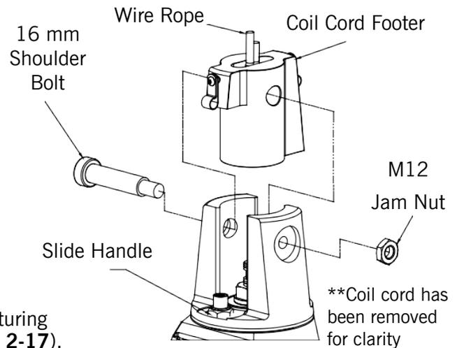
**Diagram 2-17.** Slide Handle, Shoulder Bolt and Coil Cord
