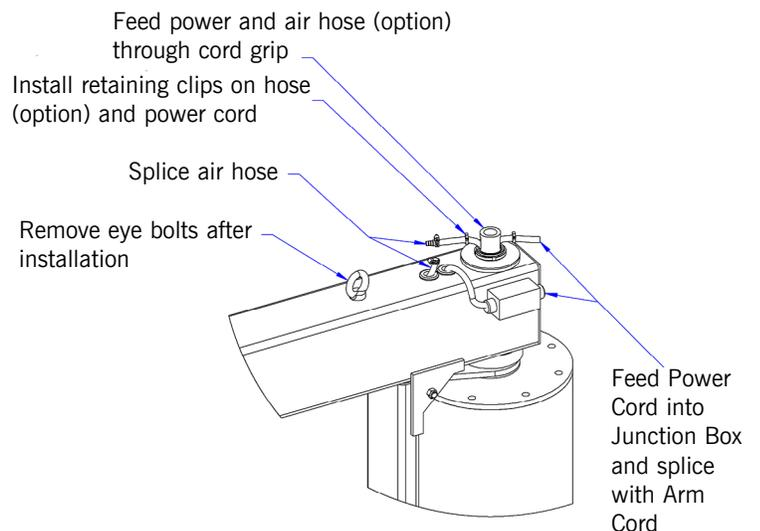
**Diagram 2-13.** Installation Electrical Connector.
