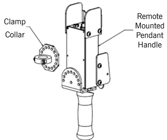
**Diagram 2-26.** Remote Mounted Pendant Handle with Collar Clamp Mounting Bracket (option)
