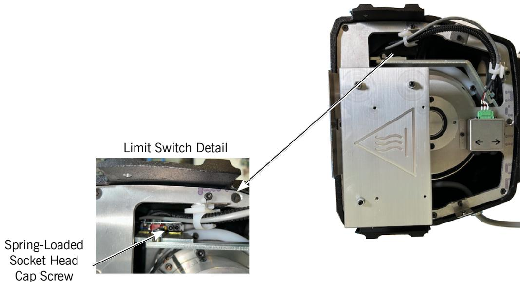
**Diagram 7-5.** Limit Switch and Socket Head Cap Screw.
