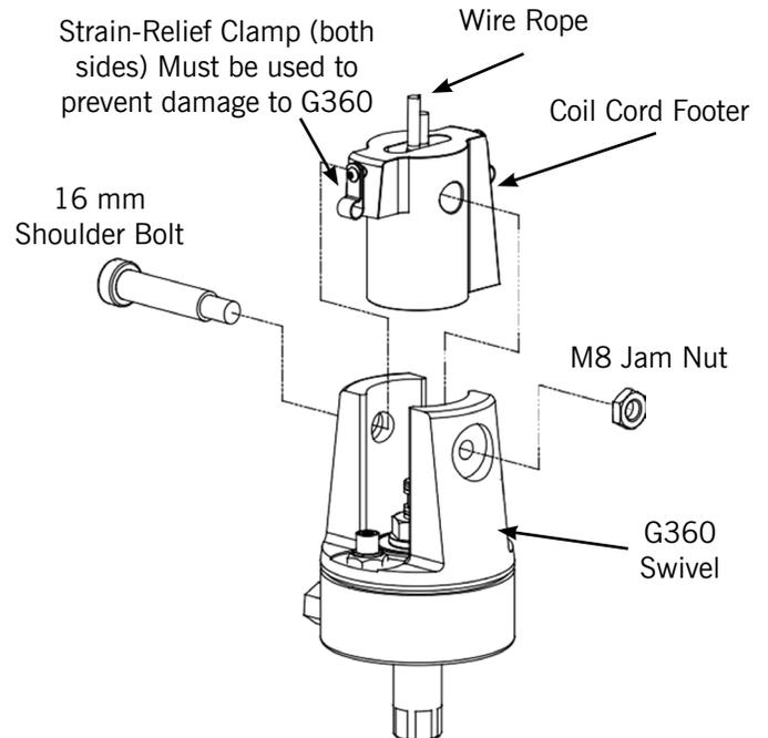
**Diagram 2-25.** G360™, Shoulder Bolt and Coil Cord.
