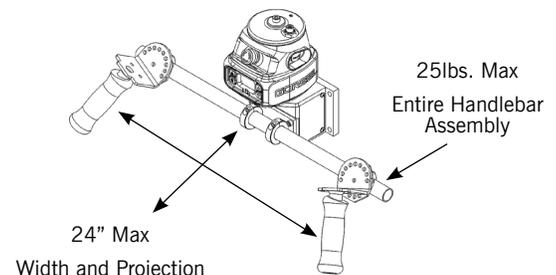
**Diagram 2-32.** Handlebar Dimensions.
