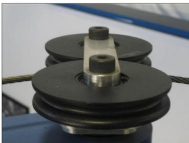
**Diagram 7-6.** Knuckle Pulley
