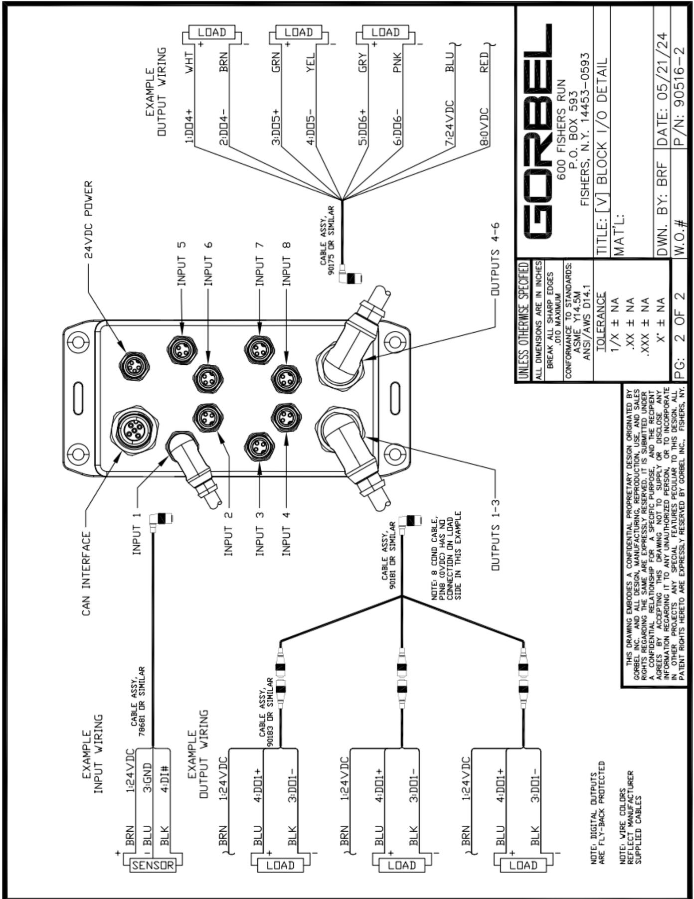
Diagram 4B-31. Expansion Block Connectors and Pin Outs.
