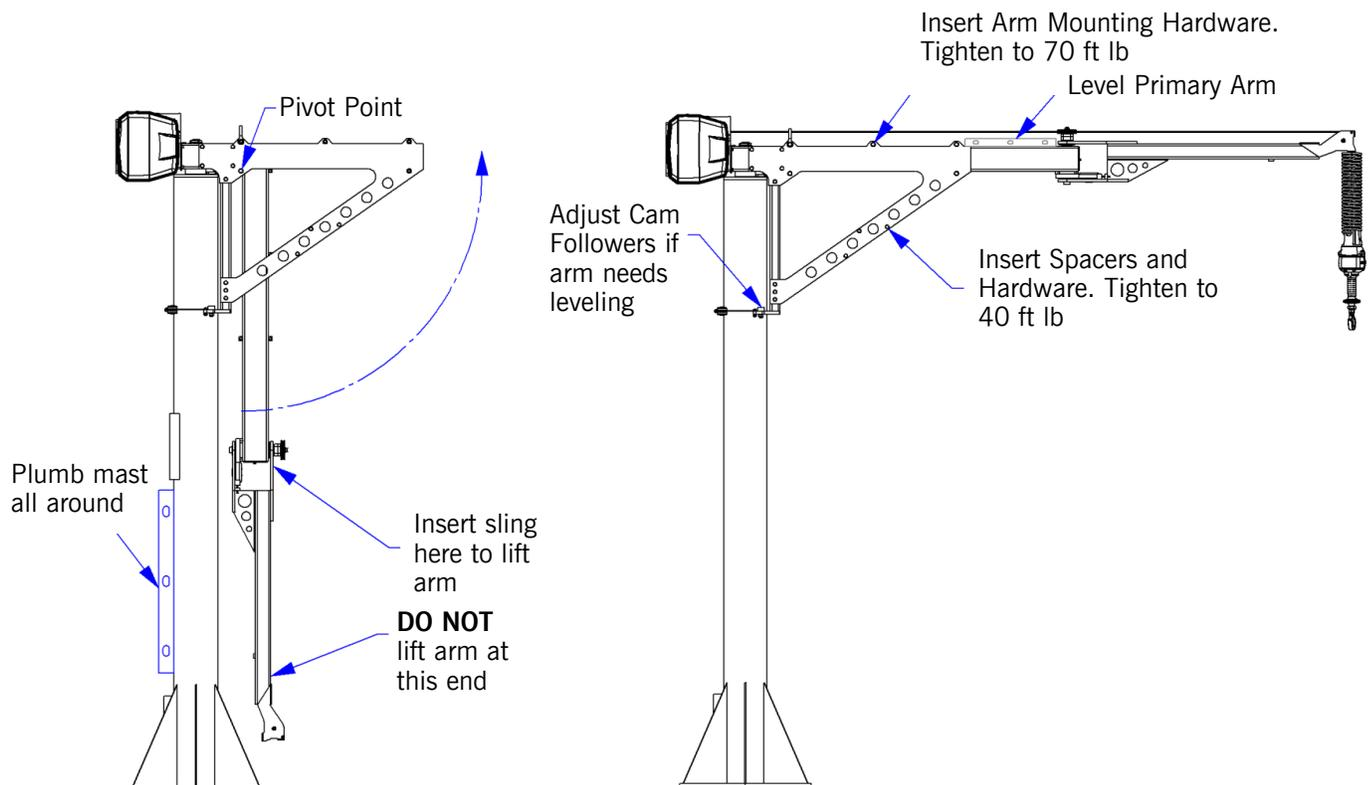
**Diagram 2-10.** Final Arm Assembly Installation.
