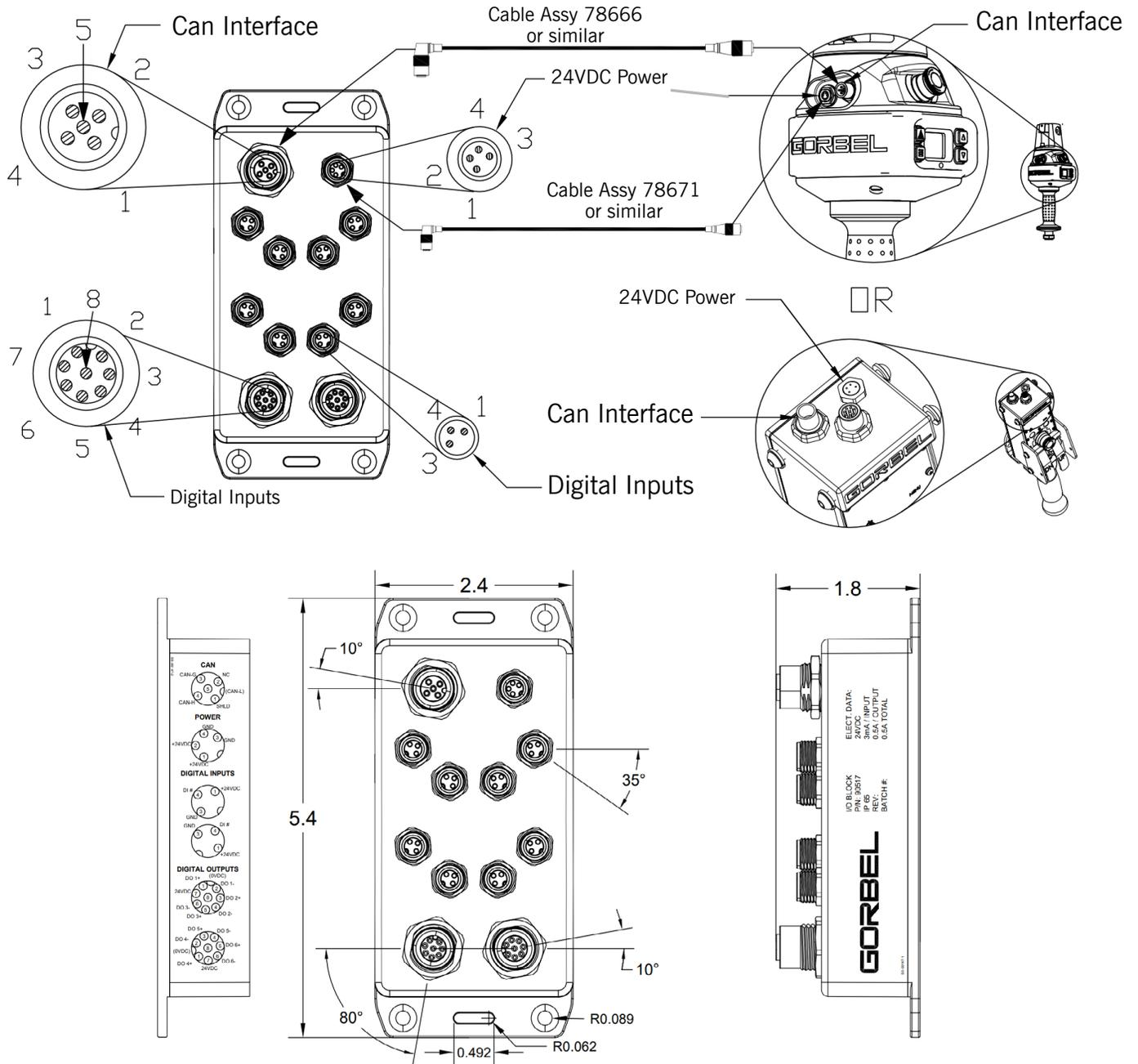
Diagram 4B-26. Handles Input/Output Block.
