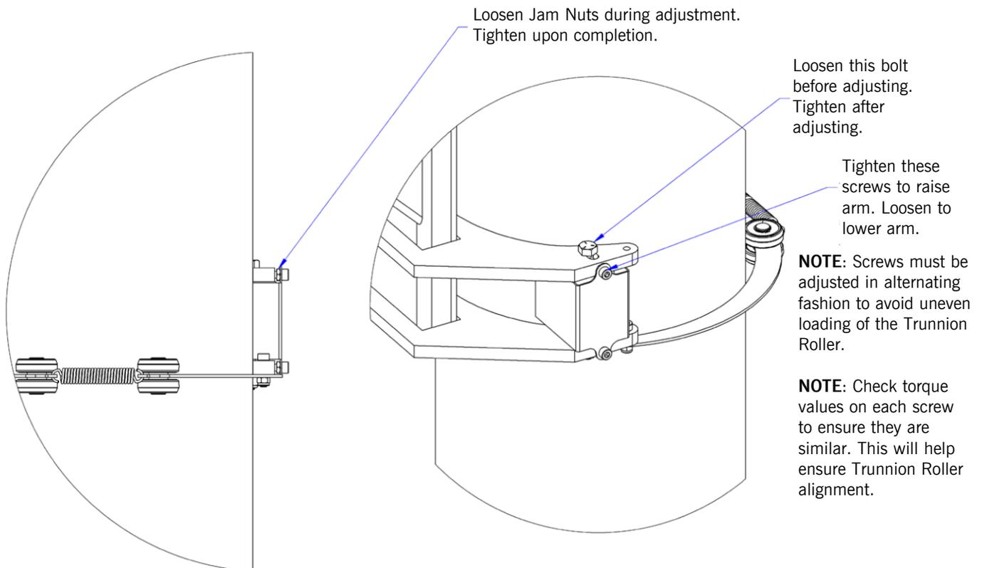
**Diagram 2-14.** Trunnion Roller Adjustment.
