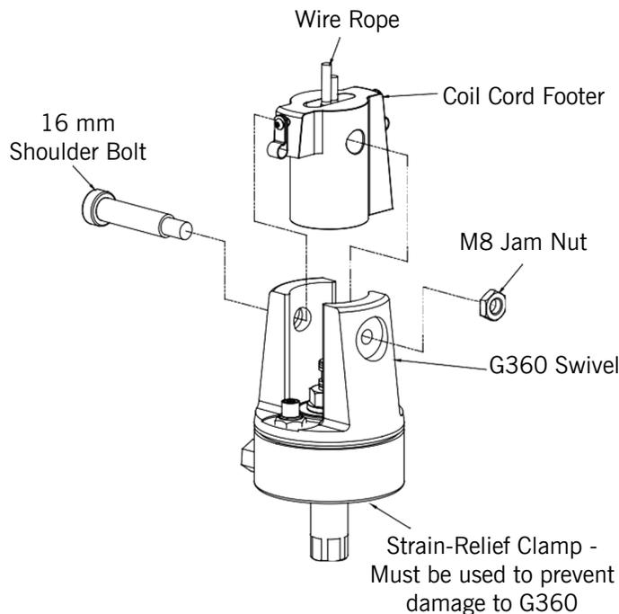
**Diagram 7-2.** Removing Wire Rope from the Slide Handle/G360.
