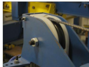
**Diagram 7-7.** Pulley Block - End of Arm
