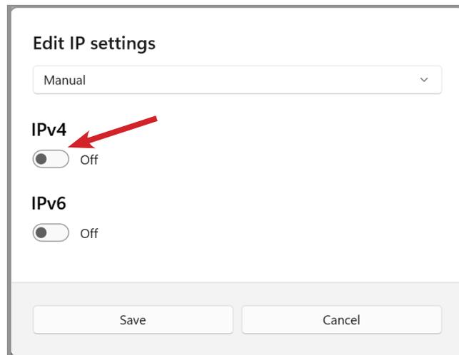
**Diagram 4B-9.** Edit IP Settings - Toggle IPv4 On.
