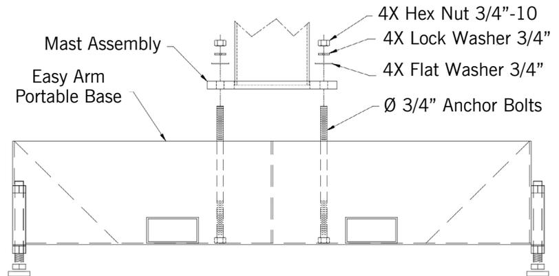
**Diagram 2-38.** Column to Portable Base Assembly.
