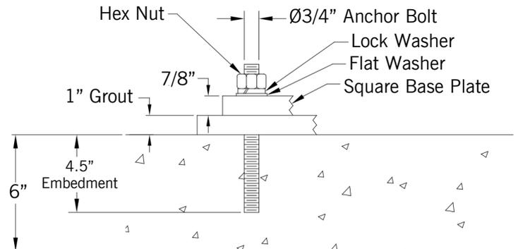
**Diagram 2-2.** Typical Square Baseplate Anchor Bolt Embedment.
