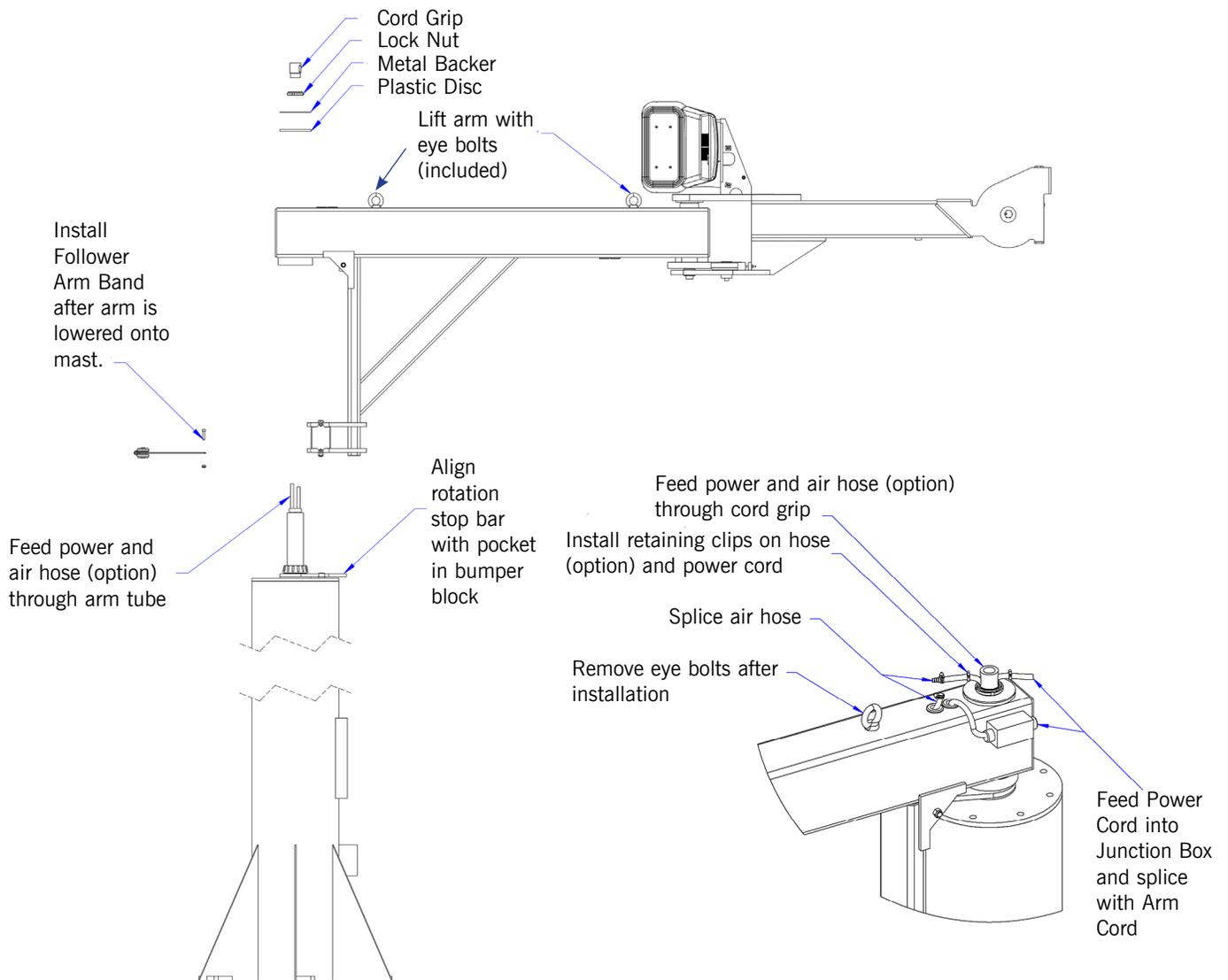
**Diagram 2-12.** Aligning Arm with Mast.
