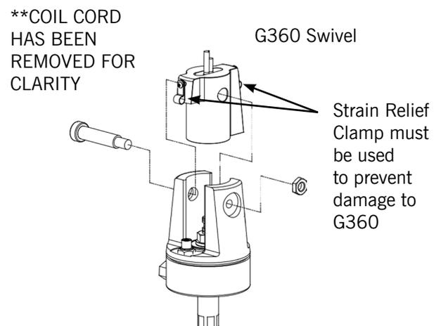
**Diagram 2-19.** G360, Shoulder Bolt and Coil Cord
