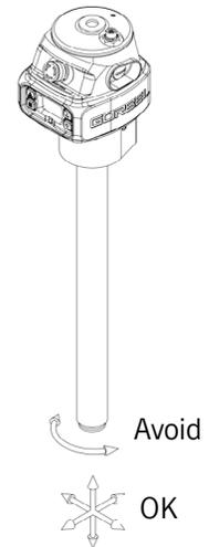
**Diagram 2-29.** Proper Use of Force Sensing Handle Grip.
