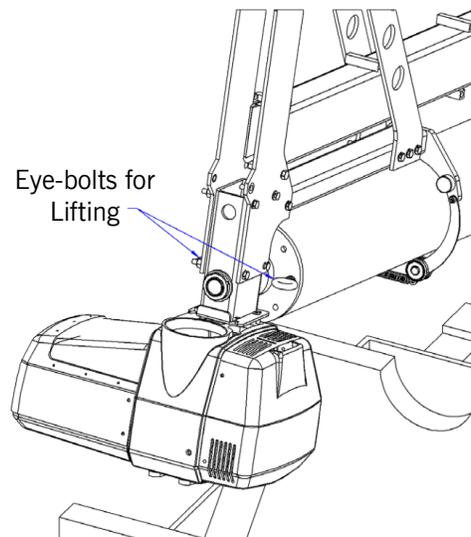
**Diagram 2-1E.** Eye-bolts for Lifting.
