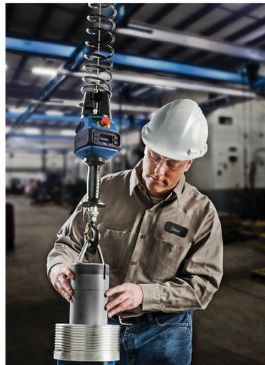
↑ In Float Mode, the operator moves the load up or down by pushing on it, rather than the Handle.
