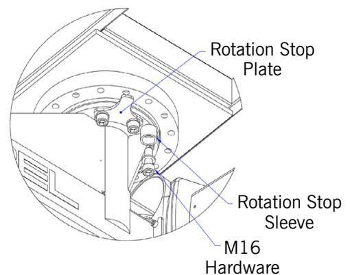
**Diagram 2-36.** Under-Hung Rotation Stop Installation.
