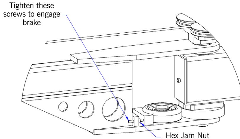
**Diagram 2-34.** Secondary Arm Friction Brake Adjustment.
