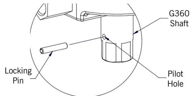
**Diagram 2-26.** Tooling Installation.
