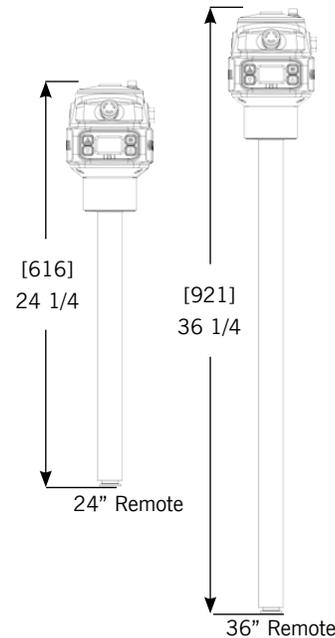
**Diagram 2-27.** Force Sensing Handle Bracket Sizes.
