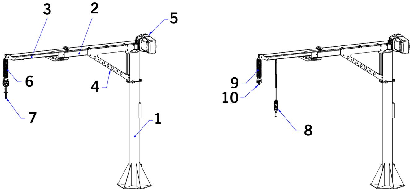
**Diagram 1-1.** Floor Mounted Easy Arm Main Components
