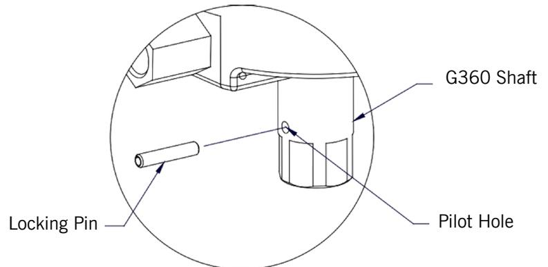
**Diagram 2-20.** Tooling Installation.
