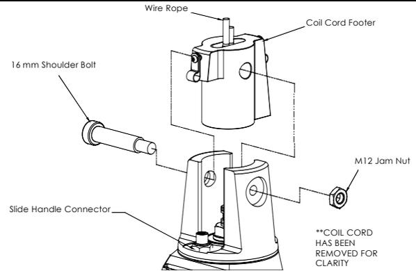
footer and wire rope to slide down into the slide handle swivel.
