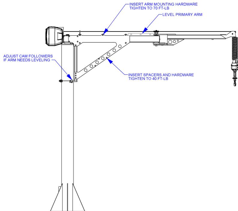
Diagram 4B. Arm assembly-leveling adjustment.
