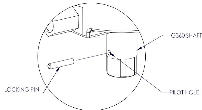
**Diagram 6D2.** Tooling Installation.
