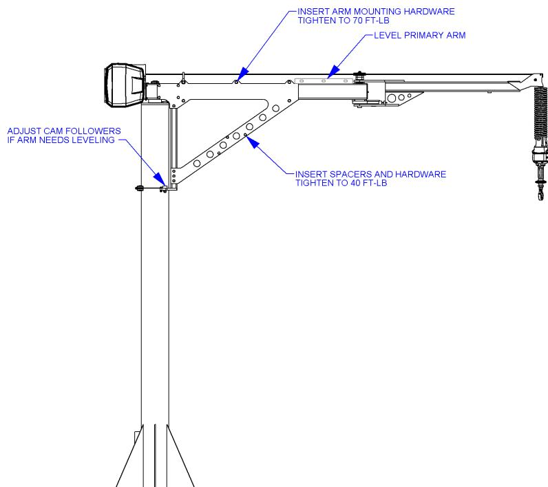
Diagram 4B. Arm assembly-leveling adjustment.
