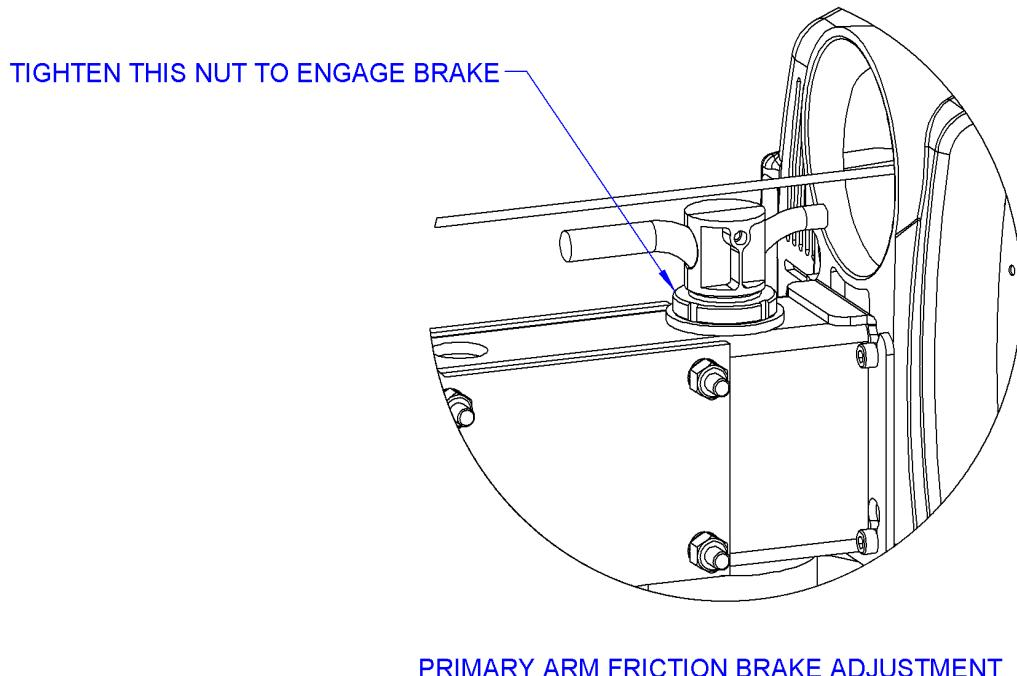
Diagram 8A. Primary arm friction brake adjustment.
