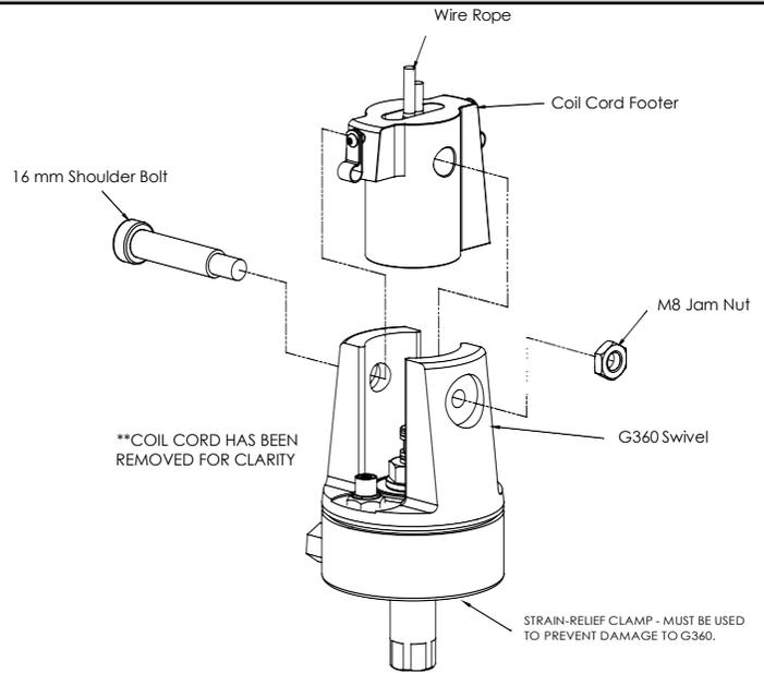
**Diagram 6D1.** G360™, Shoulder Bolt and Coil Cord.
