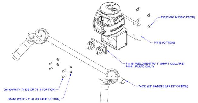
**Diagram 6F1.** Mounting handlebar and mounting plate.
