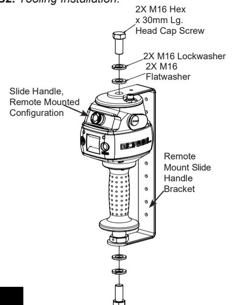
**Diagram 6B3. Remote Mounted Slide Handle, Exploded View**
