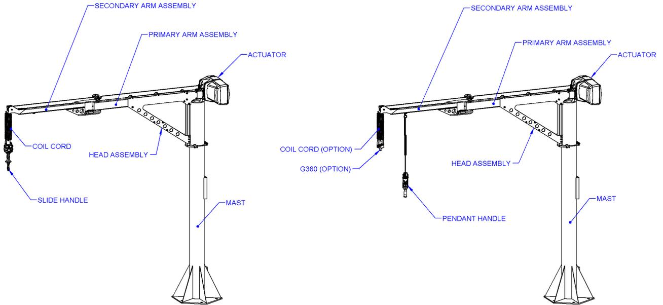
Diagram 1A. Main Floor Mounted Easy Arm® Components.
