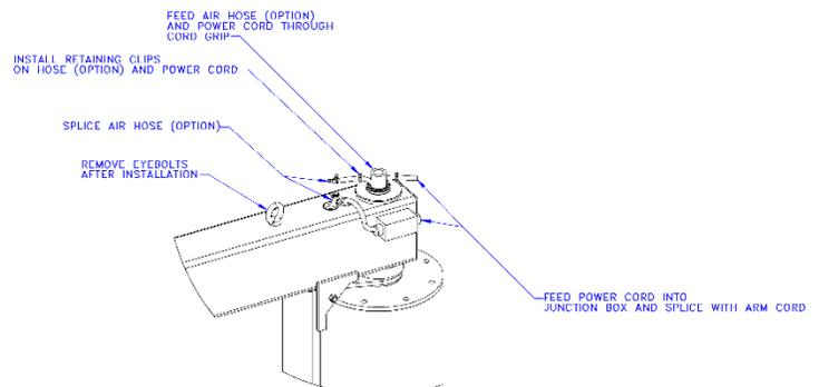
Diagram 4D. Installing electrical connector.
