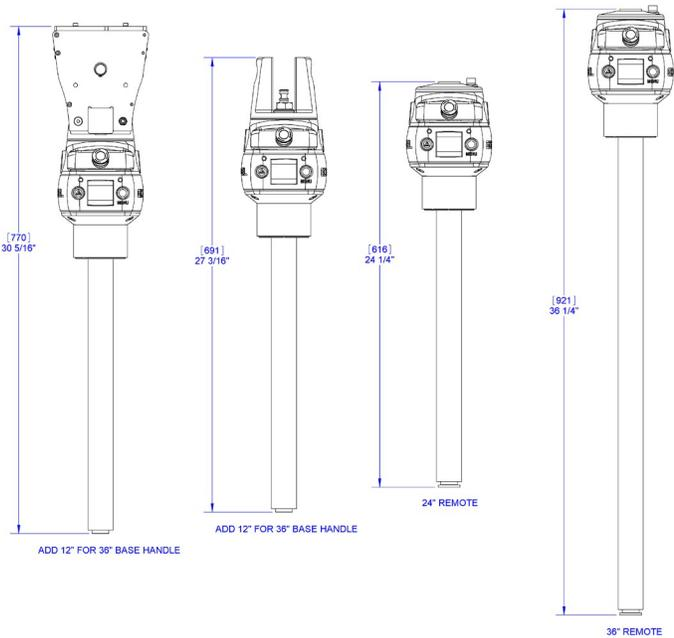
**Diagram 6E1.** Force Sensing Slide Handle bracket sizes.
