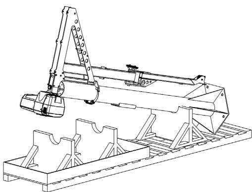
*Diagram 2D. Easy Arm® assembly removal from packaging.*
