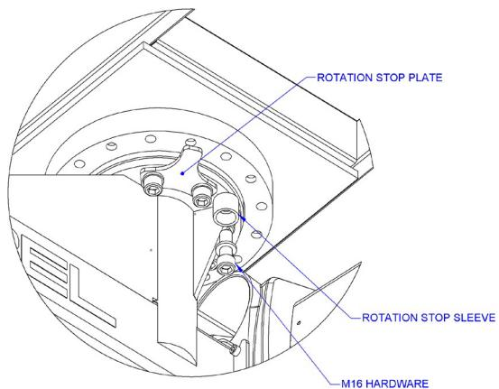
Diagram 8C. Floor mounted arm assembly rotation stop installation.
