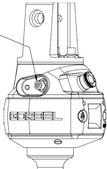
**Diagram G. Handle Input/Output Block.**
