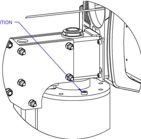
Diagram 8C. Floor mounted arm assembly rotation stop installation.
