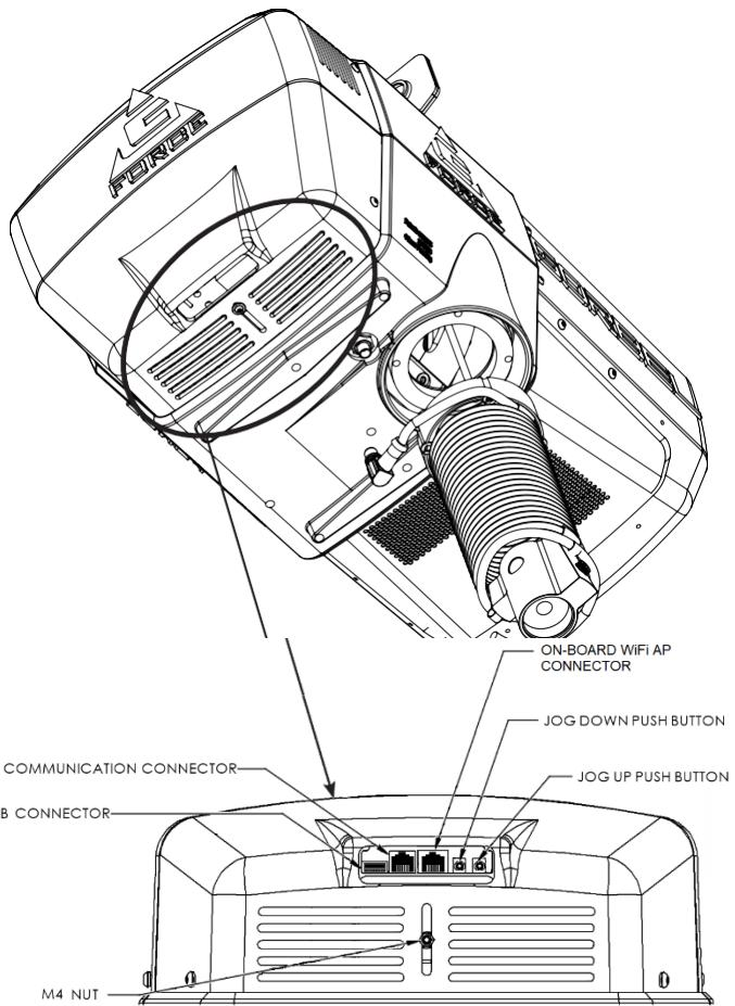
**Diagram E. Actuator - Controls Interface Display
