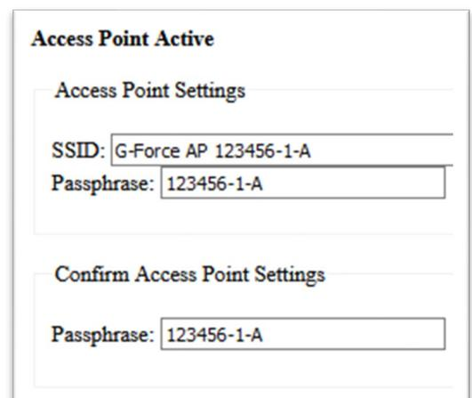
Figure 3: SSID & Passphrase setup
