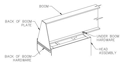
Diagram 5A. Boom Installation.
