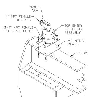
Diagram 7B. Installing top entry collector.
