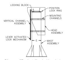
Diagram 7D. Installing locking device.
