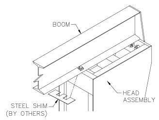
Diagram 5B. Shimming boom.
