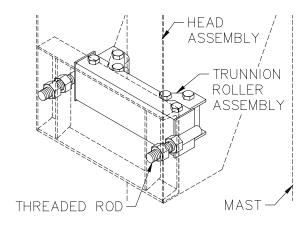
Diagram 5C. Adjusting trunnion roller assembly.
