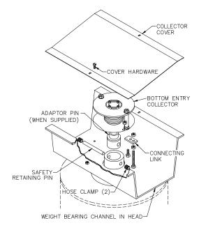
Diagram 7A. Installing bottom entry collector.
