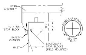
Diagram 7C. Installing rotation stops.
