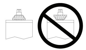
Diagram 4A. Bearing Orientation.
