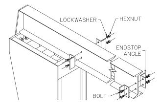
Diagram 6A. Endstop installation.
