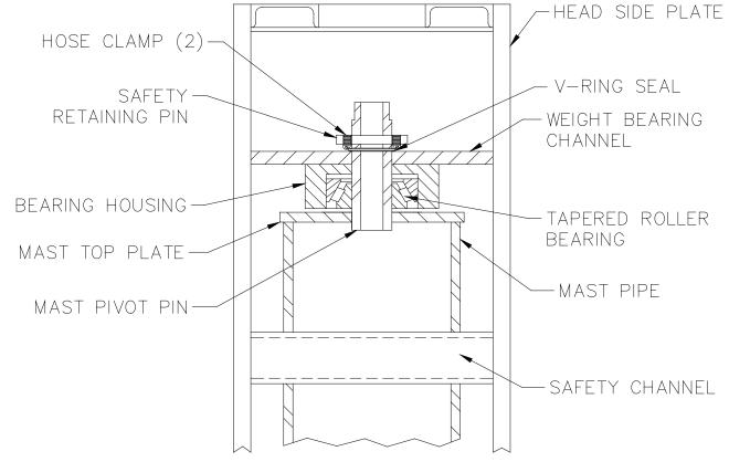
Diagram 4B. Head Assembly Installation.
