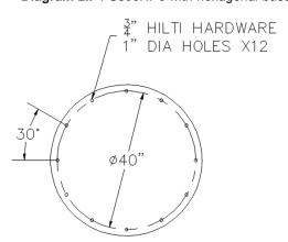
Diagram 2J. 44" dia. 12 bolt base bolt pattern
