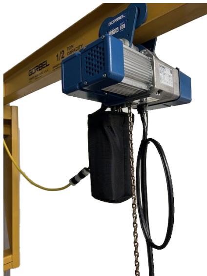
Diagram 4-8. Plugging in the Hoist.
