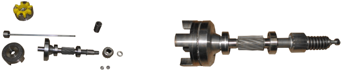
Diagram 6-19. Sliding Clutch Disassembled (l) and Assembled (r).
