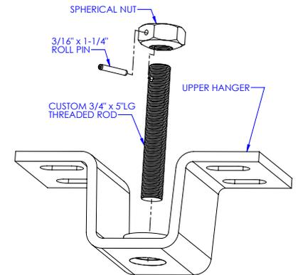
**Diagram 5A.** Assembling threaded rod to upper hanger.
