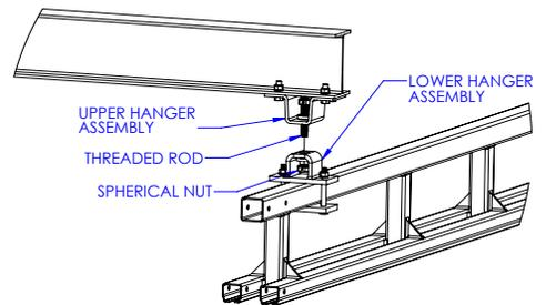
**Diagram 5D.** Attaching monorail to cantilever.
