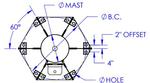
**Diagram 3B.** 12 bolt base bolt pattern.
