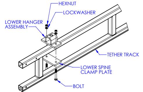
**Diagram 5C.** Attaching lower hanger assembly to monorail.
