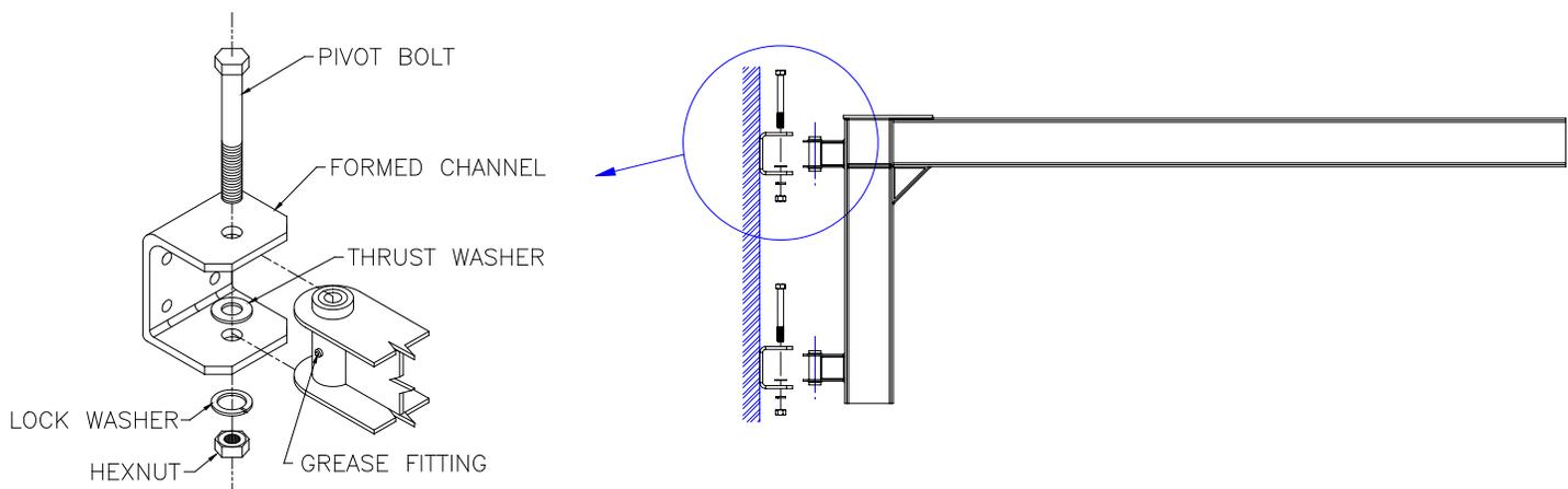
**Diagram 2B.** Attaching cantilever assembly to formed channel.
