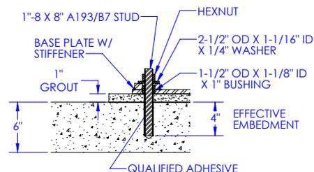
**Diagram 3D.** Anchor bolt installation.
