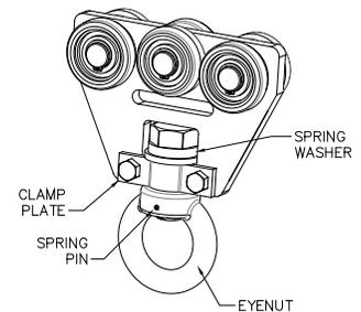
**Diagram 6A.** Tether Track® trolley installation.
