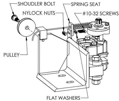
**Diagram 7C.** Assembling spring seat and pulley to bracket.
