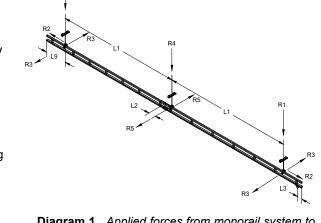
Diagram 1. Applied forces from monorail system to supporting structure.
