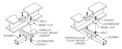
Parallel Flush Mounted Perpendicular Flush Mounted **Diagram 3B.** Attaching flush mounted hangers to building support beam.
