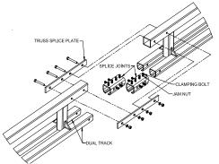
Diagram 4C. Splicing dual trussed track.
