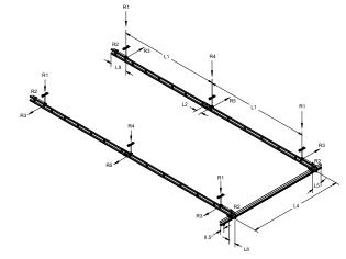
**Diagram 2.** Applied forces from bridge to supporting structure.
