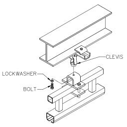
Diagram 3C. Attaching flush mounted sloped ceiling hangers to top hanger assembly.
