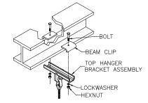
**Diagram 2E.** Bolting standard top hanger bracket and beam clips to existing support beam.
