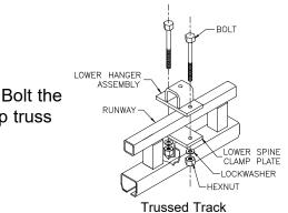
**Diagram 2H.** Bolting lower hanger assembly and spine clamp plate to trussed track.
