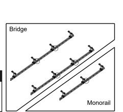
Diagram 3F. Installing end stop.
