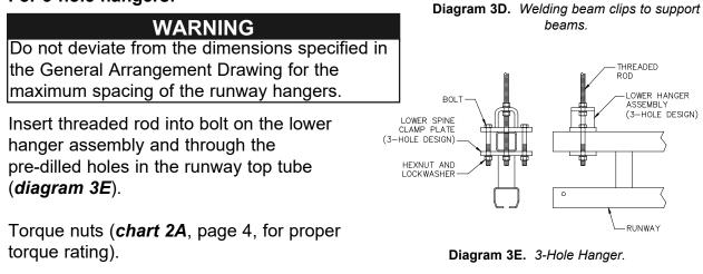
• IMPORTANT: Note the placement of the threaded rod hardware in *diagram 3E*. The lower hanger assembly and the truss top tube must be properly clamped to provide adequate support.
