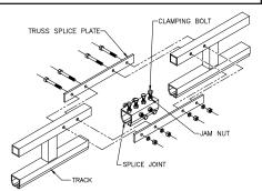
Diagram 4B. Splicing trussed track.
