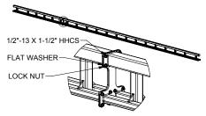
Diagram 4D. Plate style splice joint detail.
