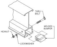
Diagram 5C. Installing end stop.
