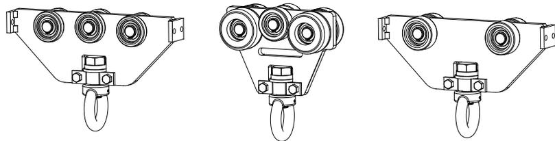
Diagram 6B. Various monorail and bridge trolley configurations.
