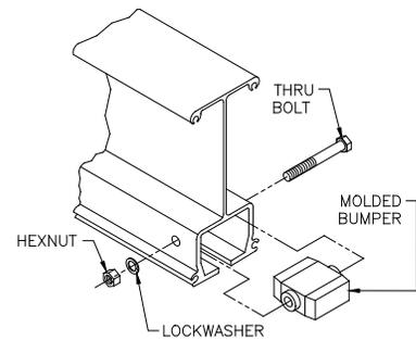
Diagram 5C. Installing end stop.
