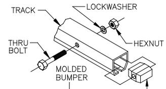
Diagram 5D. Installing end stop.
