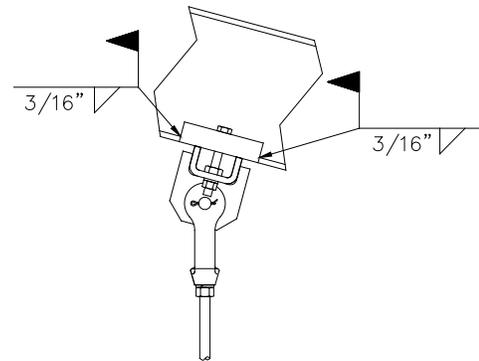
Diagram 3D. Welding beam clips to support beams.
