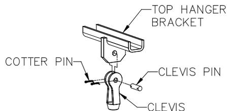
Diagram 2B. Attaching clevis to top hanger bracket.
