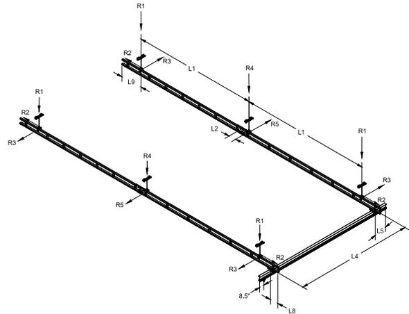
**Diagram 2.** Applied forces from bridge to supporting structure.
