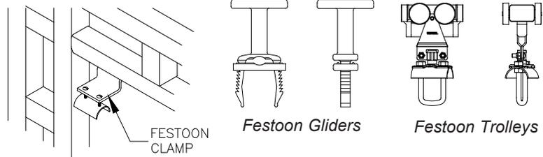
Diagram 5A. Installing festoon clamp and festoon gliders/trolleys.
