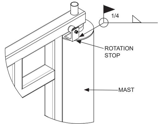
Diagram 9C. Welding rotation stops on the WSJ360.
