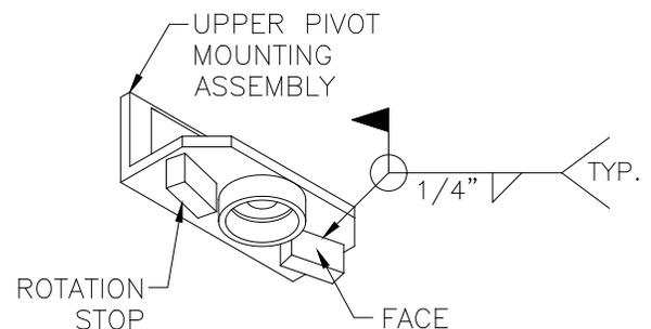
Diagram 9D. Welding rotation stops on the WSJ200.
