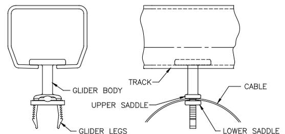
**Diagram 6A.** Installing electric cable on festoon glider.
