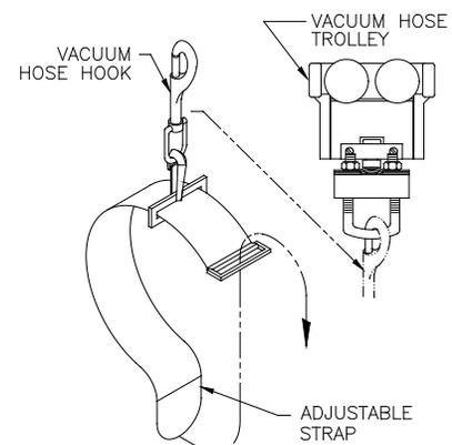
**Diagram 6C.** Installing hose on vacuum hose trolley.
