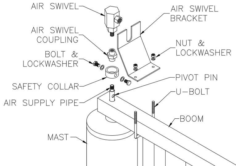
**Diagram 9B.** *Installing bottom entry air swivel assembly.*
