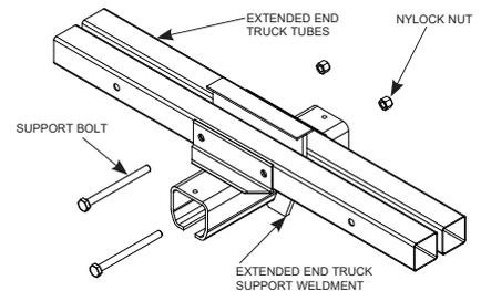
**Diagram 5F.** Assembling extended end truck.
