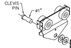
**Diagram 6C.** Installing hoist on 1000-2000# hoist trolley.
