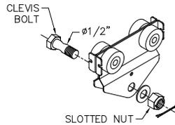
**Diagram 6A.** Installing hoist on 150-250# hoist trolley.
