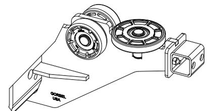
**Diagram 5E.** Installing tow arm spacer on end truck.
