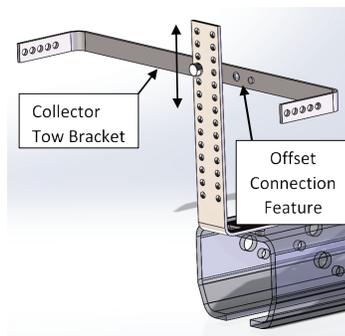
**Diagram 10Q.** Tow bracket directly mounted to mast.
