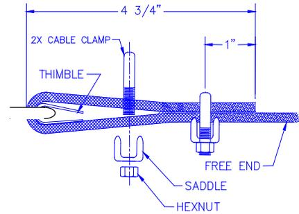
**Diagram 11A.** Saddling the cable on one end.
