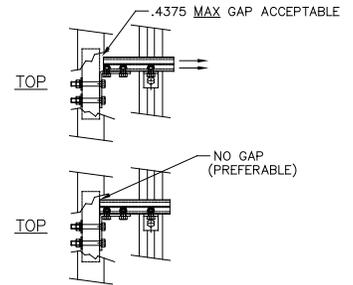
5. A gap of approximately 0.25" will exist between the mounting bracket and track spine surface due to vertical tube fillet welds (0.25" high). Hanger assemblies are to be located as close to the steel track spine as possible barring these welds (**diagram 10H**).
