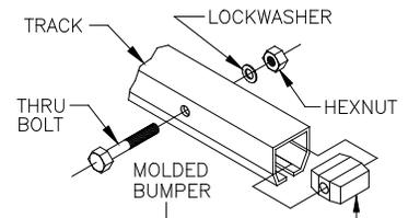
**Diagram 8C.** Installing end stop on runway/monorail/festoon stack section.
