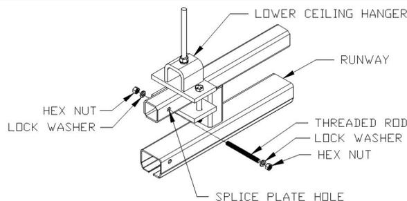
Diagram 3E. Hanger Retaining Bolt, 250#-2000#.
