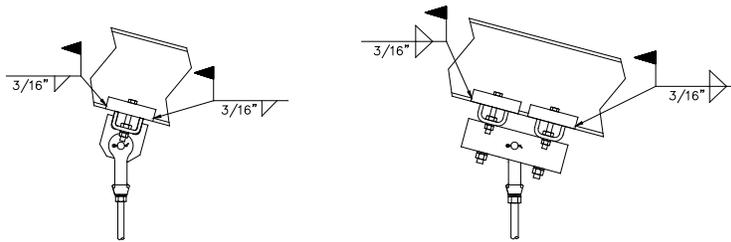
Diagram 3D. Welding beam clips to support beams.
