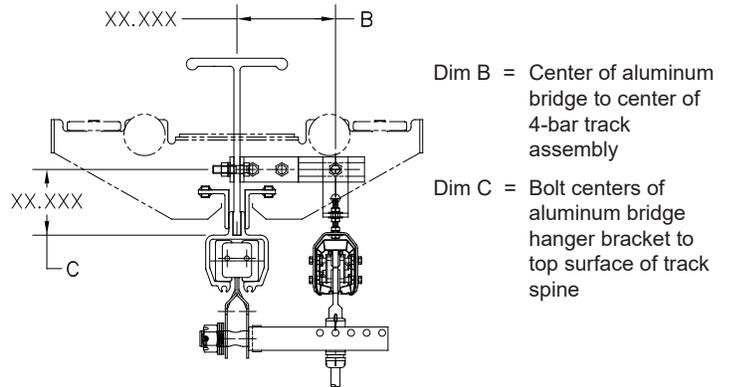
**Diagram 10J.** Two piece aluminum bridge B-C dimensions.
