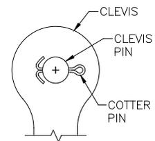
**Diagram 2C.** Installing cotter pin through clevis pin.
