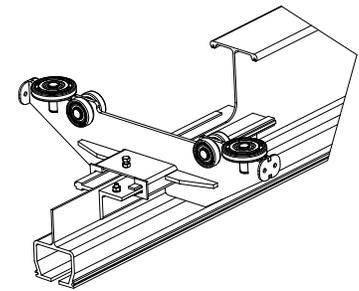
**Diagram 5C.** Installing clamping end truck on coped aluminum bridge.
