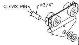
**Diagram 6B.** Installing hoist on 500# hoist trolley.
