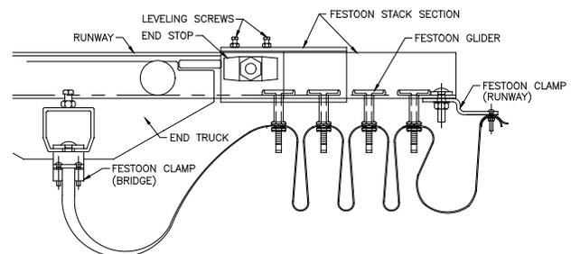
**Diagram 8D.** Installing electric cable on festoon glider.
