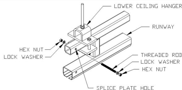
Diagram 3E. Hanger Retaining Bolt, 250#-2000#.
