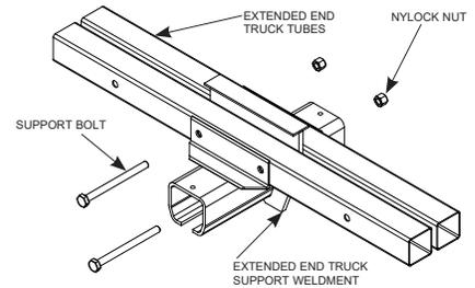
**Diagram 5F.** Assembling extended end truck.
