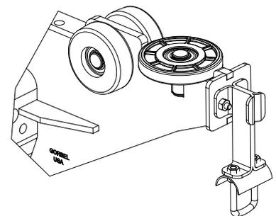
**Diagram 5D.** Installing tow arm on end truck.
