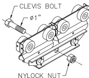
**Diagram 6G.** Installing hoist on loadbar hoist trolley.
